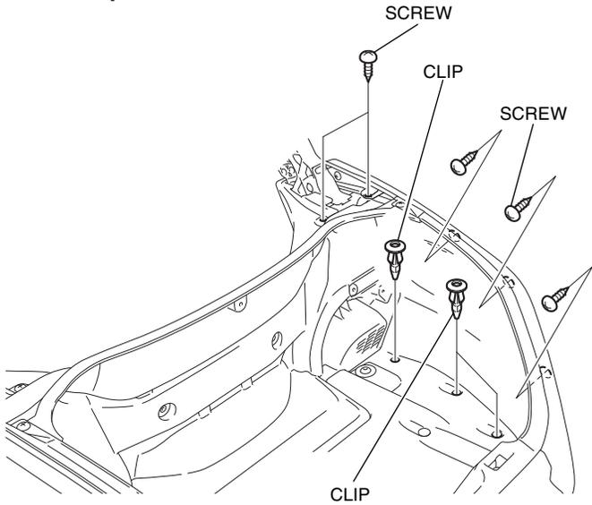
11. Remove the trunk right side cover as shown.
