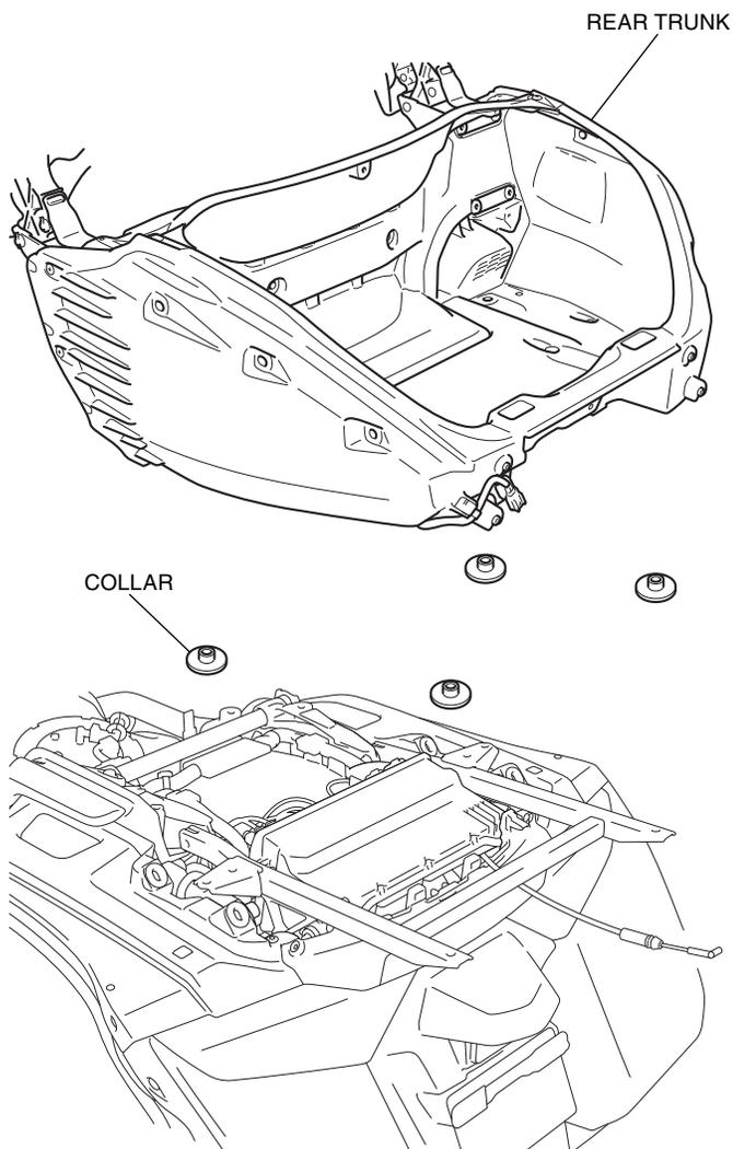
21. Drill at the marked line of the rear trunk as shown.
