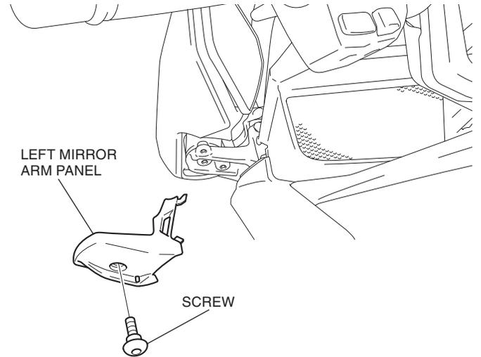
7. Remove the left rear view mirror as shown.
