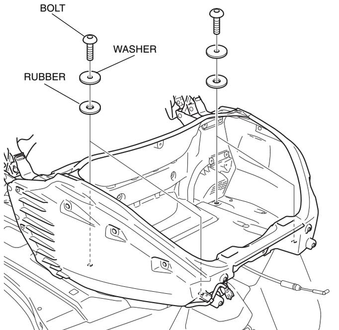
20. Remove the rear trunk and collars as shown.
