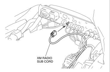
39. Route and connect the XM radio antenna cord as shown.
