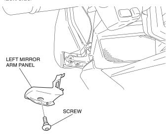
11. Remove the left rear view mirror as shown.
