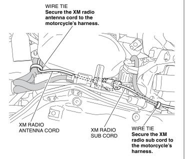
42. Secure the XM radio sub cord with the wire ties as shown.
