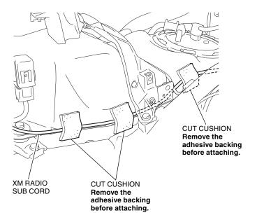
46. Secure the XM radio sub cord with the wire ties as shown.
