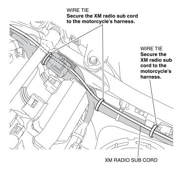
47. Secure the XM radio sub cord with the wire tie as shown.
