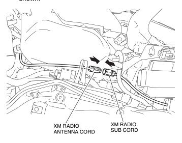
40. Secure the XM radio antenna cord with the wire ties as shown.
