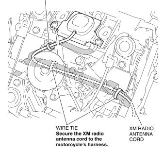
41. Secure the XM radio antenna cord and XM radio sub cord with the wire ties as shown.
