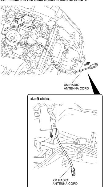
29. Route the XM radio sub cord as shown.Left side view, without top shelter for clarity>
