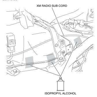
45. Secure the XM radio sub cord with the cut cushions as shown.
