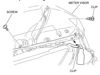
25. Remove the meter visor as shown.
